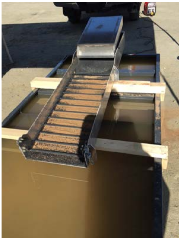
Photo 26. A modern-day sluice box made from aluminum to keep it light. Photo by the author.
