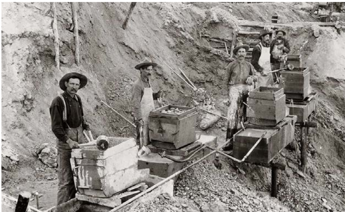
Photo 28. Operation of rocker boxes that required much less water than sluicing. Water is added from pots, as the man on the left just has done. Photo historycollection.ca. (Bildern något beskuren)
