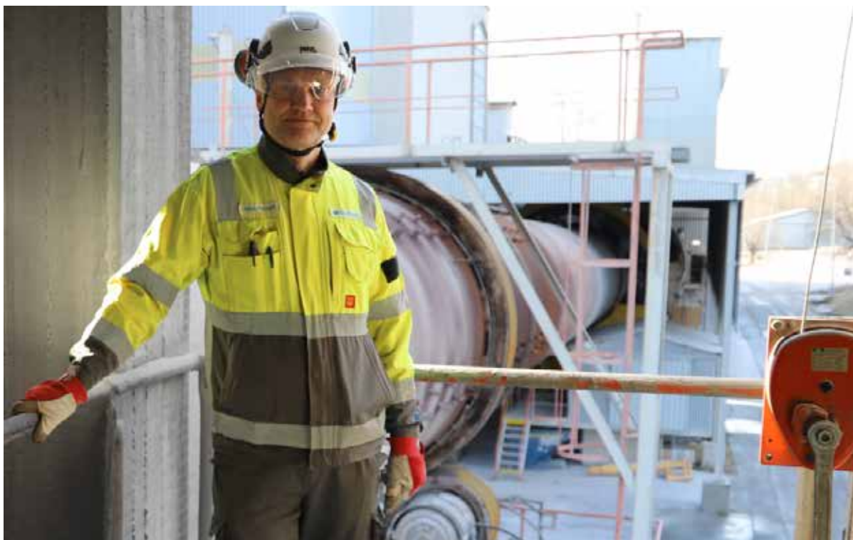
Surplus heat from lime kilns is supplied to the district heating company of the city of Lohja. The surplus heat supplied by Nordkalk is enough to heat about 1,000 detached houses. The picture shows the kiln production manager Esko Niemelä next to the rotary kiln.
